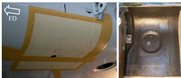
Figure 5-4: Repair Finished except Top Coat
