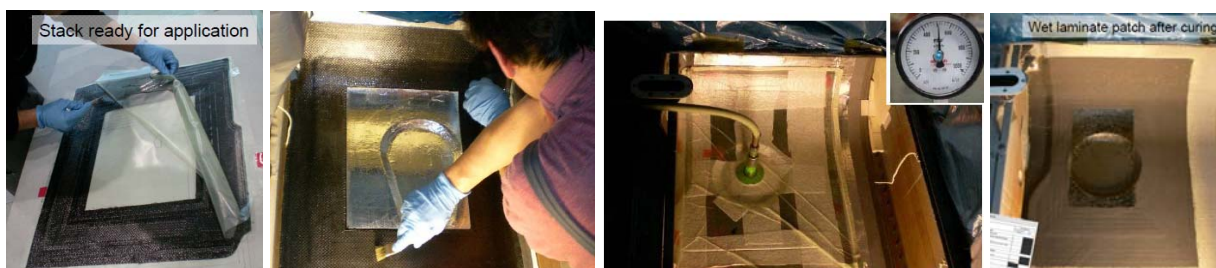
Figure 5-3: Inside Wet-Laminate Patch
